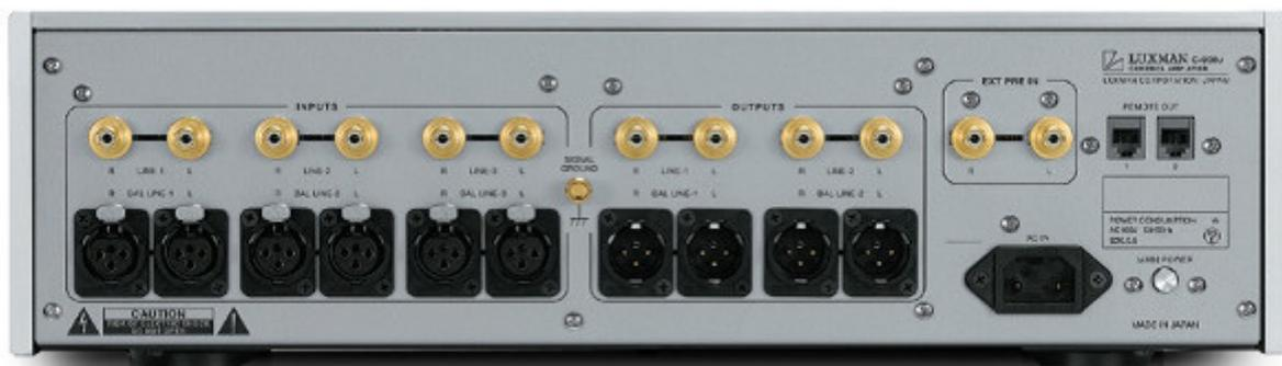
The C-900u provides usual and sufficient connectivity on its rear panel: 3 RCA inputs, 3 balanced XLR inputs, 2 RCA and 2 XLR outputs, one RCA input for a control amplifier that helps to make the Luxmans a part of AV system, and remote link connection. The main power switch is placed next to the IEC inlet - the front power button only brings the amp to STAND BY.
